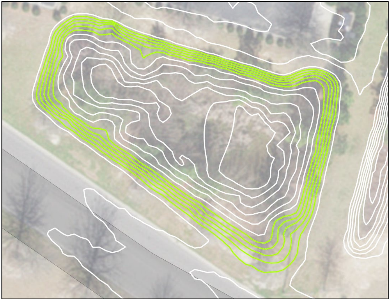
Figure 9 - Example: early prediction results. Predicted DDB contours are shown in green, with all contours in white. As seen here, early model runs evaluated individual contours instead of stacks, which resulted in multiple predicted DDBs in the same depression.
