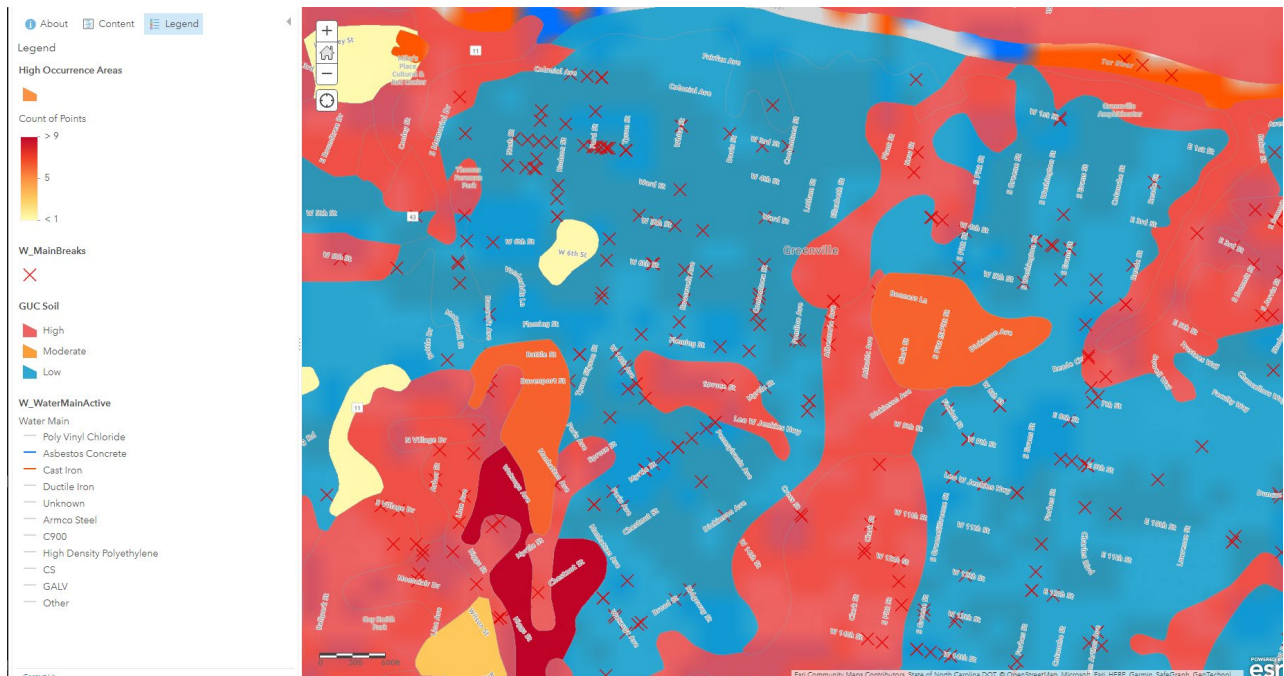
Figure 10: Water main break map illustrating the ability to use gathered information from the mobile field application to improve infrastructure planning and maintenance.
